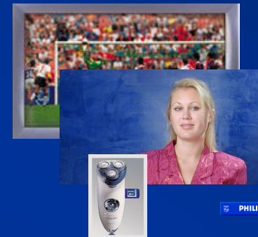
MPEG-4 – Several Objects can be sent separately and combined in decoder
